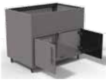
APPLIANCE SKIRT: 12" TALL 27" - 48" = 2 DOOR (LH/RH) 51" - 54" = 3 DOOR (LH/RH/RH) 57" - 66" = 4 DOOR (LH/RH/LH/RH) VENTED IN FLOOR AND BACK PANEL DOES NOT ACCOMMODATE LP TANK
